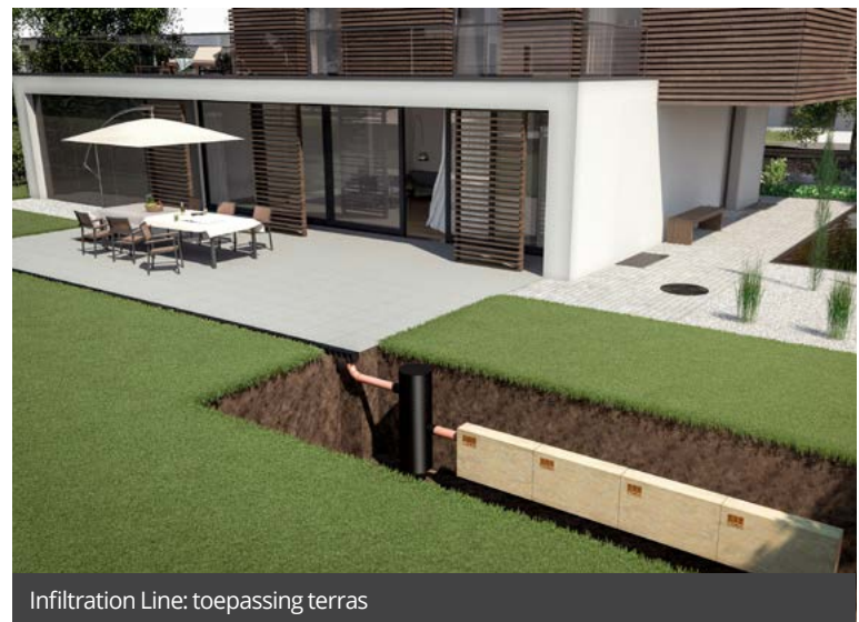
Infiltration Line: toepassing terras
